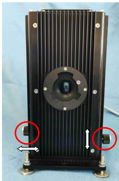
Figure 4 Lamp Housing in use since year 2022. Justage unit with 2 axis. X-X, Z-Z
