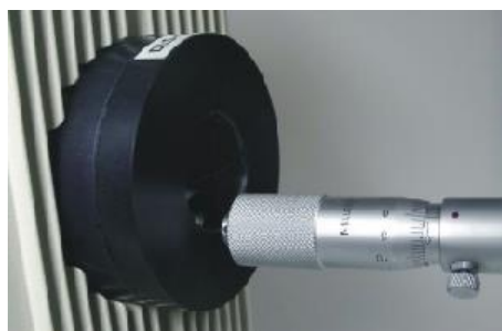
Figure 5 The alignment jig in front of the lamp. Each jig is assigned to one lamp and has to be connected so that the sign on it shows upwards. The reference point for distance measurements is below the window.
